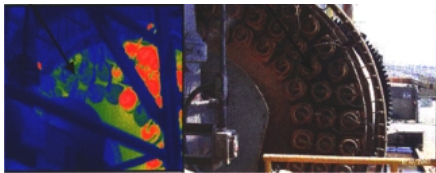
Figure 6.2.9. Inoperable steam heaters seen by cooler blue areas when compared to the operating heaters warmer red or orange colors.
