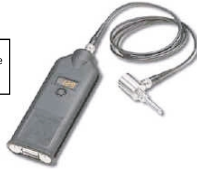
Examples of typical handheld vibration sensing meters. Note readout providing immediate level indication.
